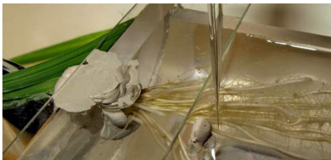
Laboratory setup with double chamber, the sensor is positioned into root cortex. Photo: Ole Pedersen
